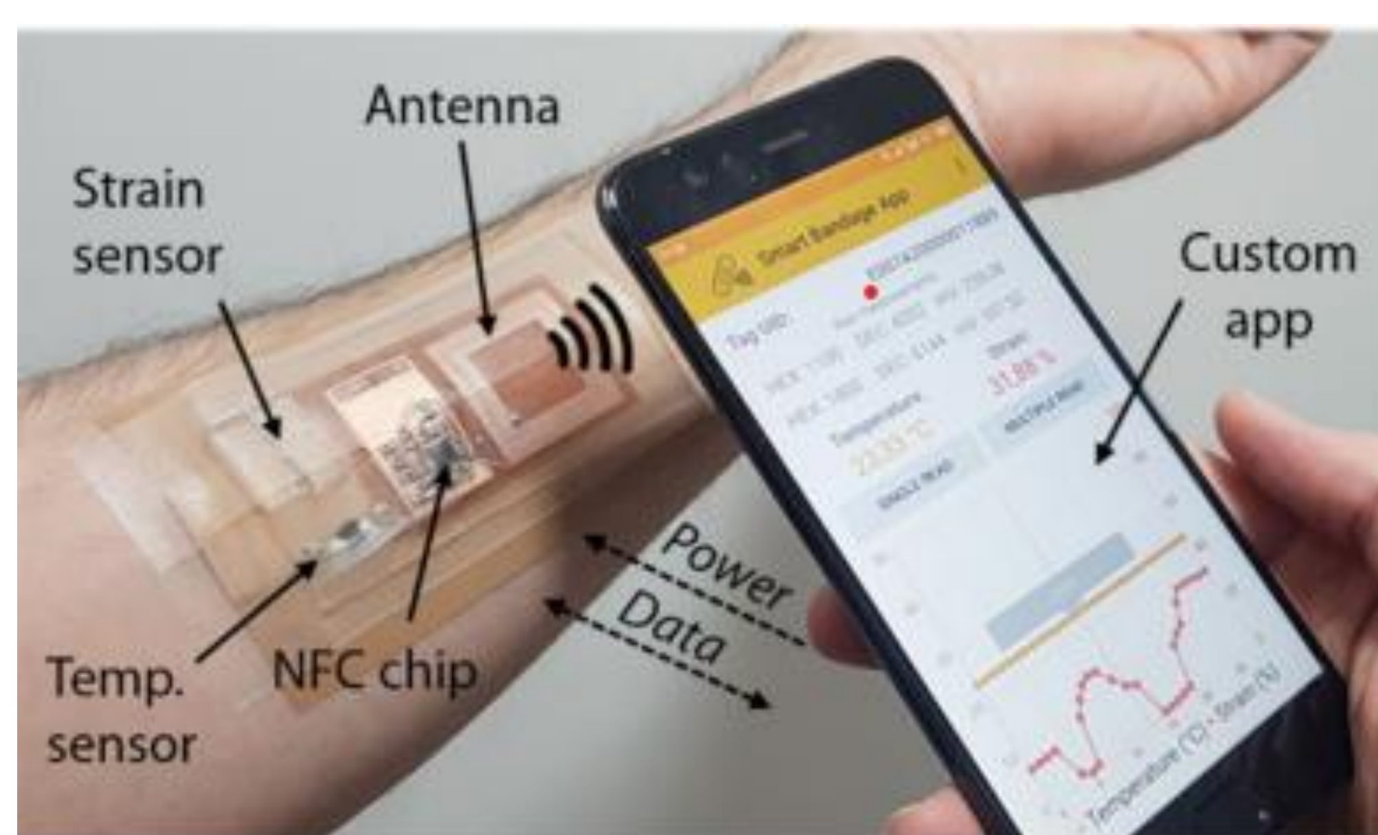
Fig. 2.3 Prototype of a smart bandage for the treatment of chronic wounds
