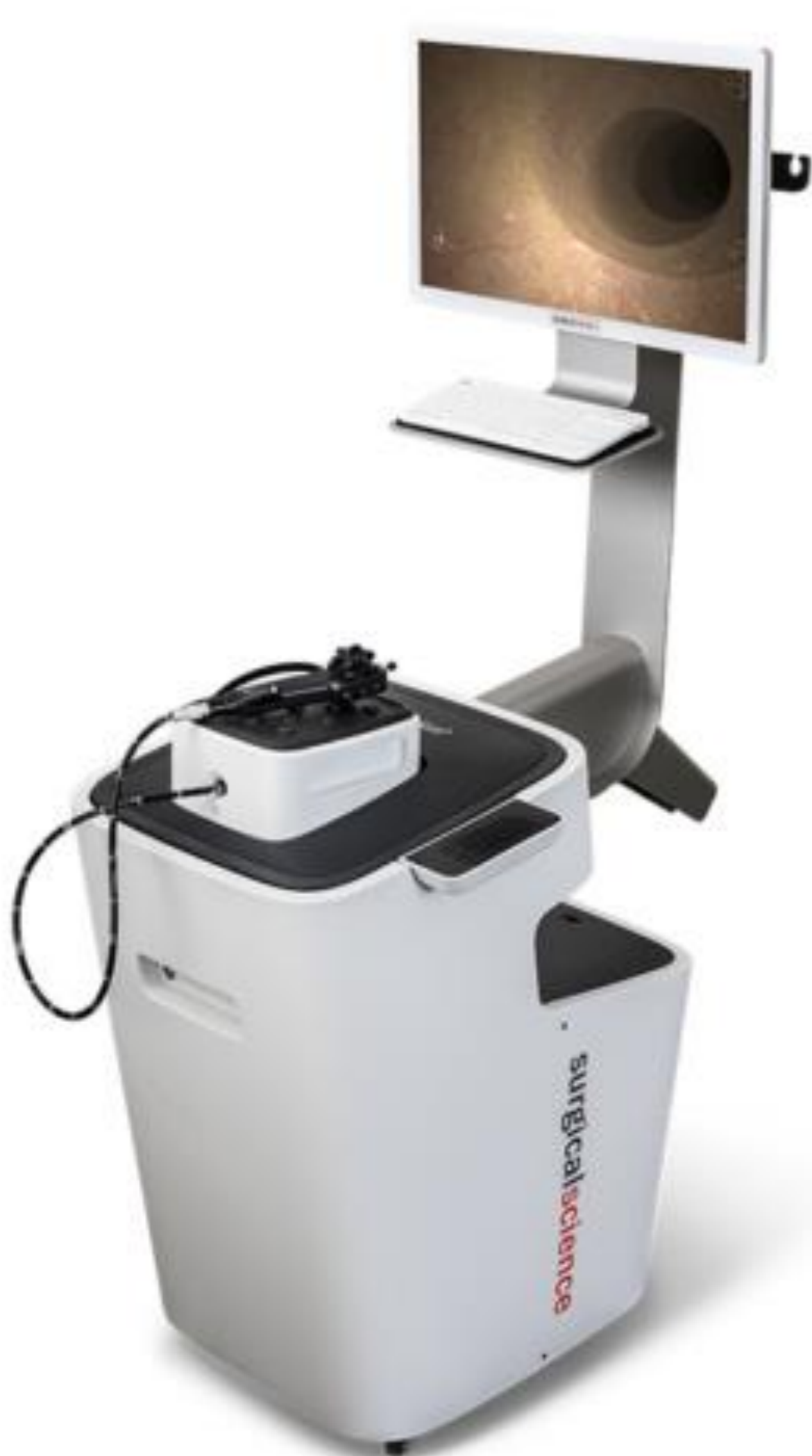
The EndoSim® VR Simulator is a virtual reality tool used in endovascular surgery training. It provides a simulated environment where trainees can practice various procedures, offering realistic scenarios and feedback.
